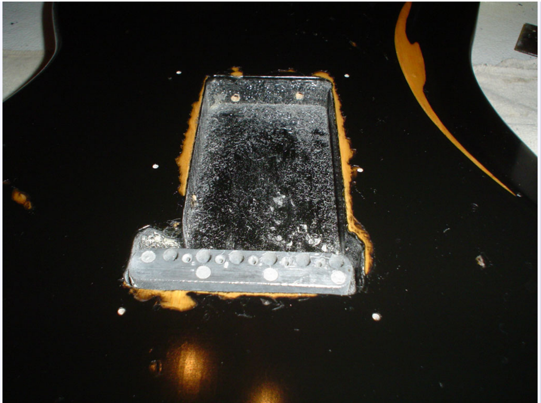
Another shot of not going thru the color coat, just thru the clear.. This is all dependent on the angle.
