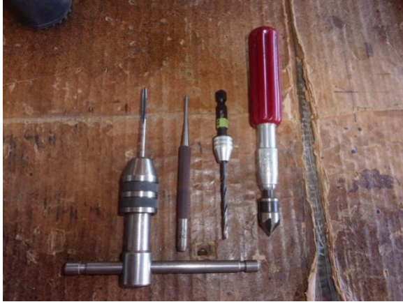
5. Threading tools. The hobby knife handle has been drilled to fit the countersink.
