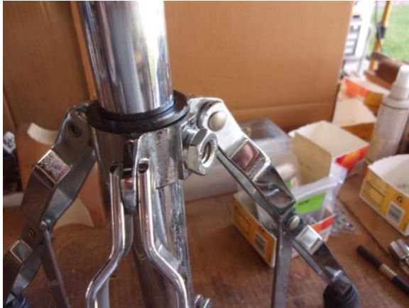
Ludwig stand with stainless insert, locking nut, and lockwasher.
