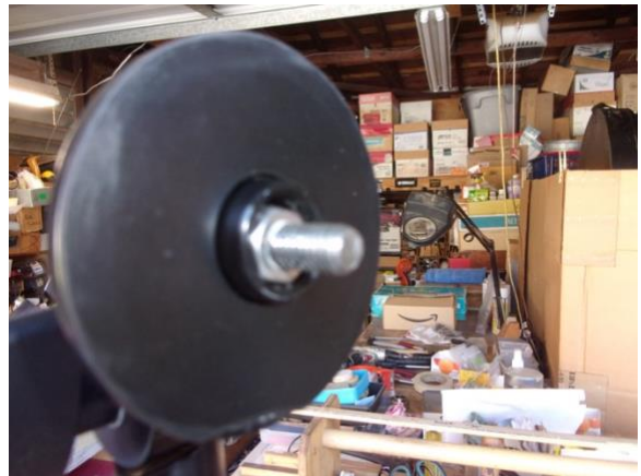
8. Incidentally, the threads on the top bolt for mounting the bass had to be chased in order to work properly.
