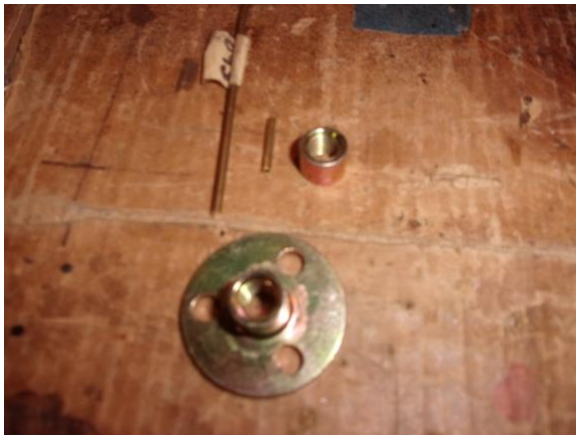
2. Making the insert. A furniture T nut was just right for this repair. The internal thread is m8-1.25 and the outer diameter is m12. The flange was cut off with a metal cutting blade (32 tpi) in a coping saw frame.
