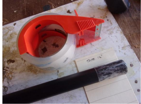
Step 8.1: Stand no. 1 needed some packing tape in two places to adapt it to the repaired stand base.
