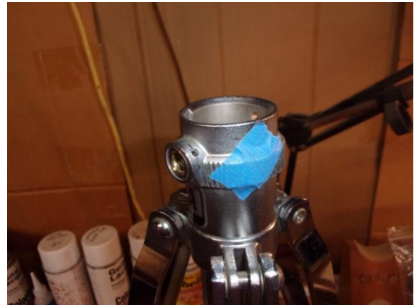
4. The insert was secured with a 6-32 brass bolt about 1/4" long. The tap hole (#36 drill) was threaded through the casting and one side of the insert. Note that I tried 3/32" pins (a rod and also a tube) and neither worked well. A spring pin would be too hard for this application. If it fouled the threads the problem could not be corrected with a tap.
