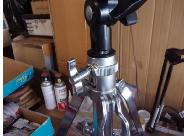
Yamaha stand with steel insert, shims, and 6-32 locking bolt.
