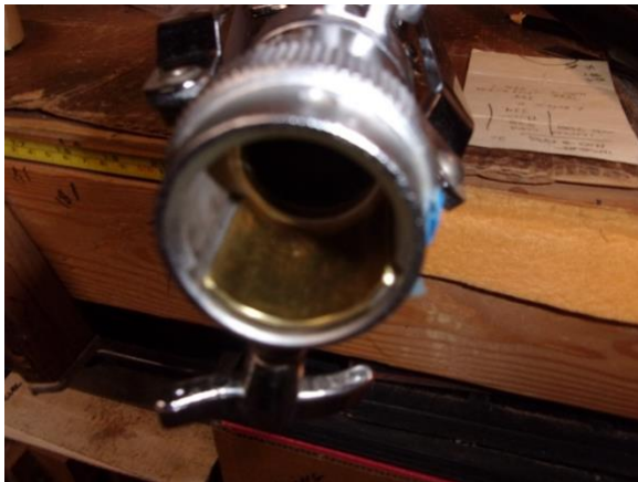
6. A new bearing plate was made and installed.
