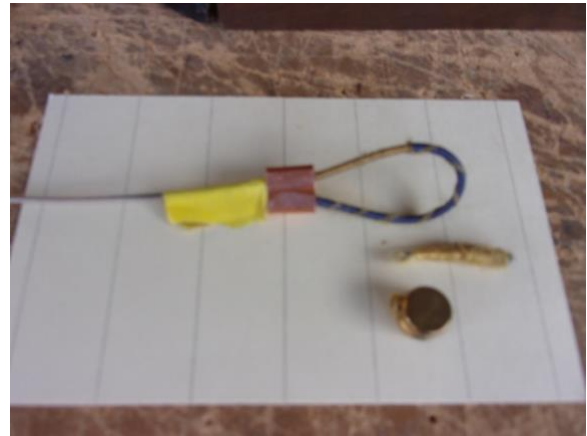
3.2 Crimped string end with loop of string, extra piece of string, old ball end.
