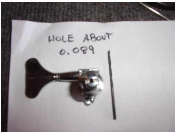
5.1 Tuner and number drill to approximate hole.
