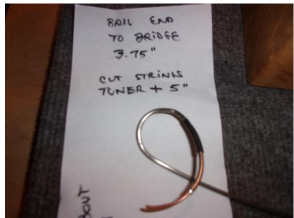
5.2 Some windings removed from the string at the tuner end. Heat shrink tubing was installed to protect the outer wrap.
