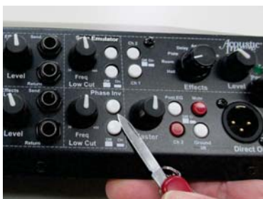
Prying out the switch cap
