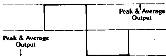
Artificially Generated Square Wave Average Output Equals Peak Output
