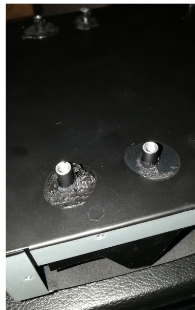
Fig. Left: back of the box before (source: tc electronic), middle: with the amplifier module detached, Right: M5 threaded sleeves and bitumen adhesive on the amplifier module
