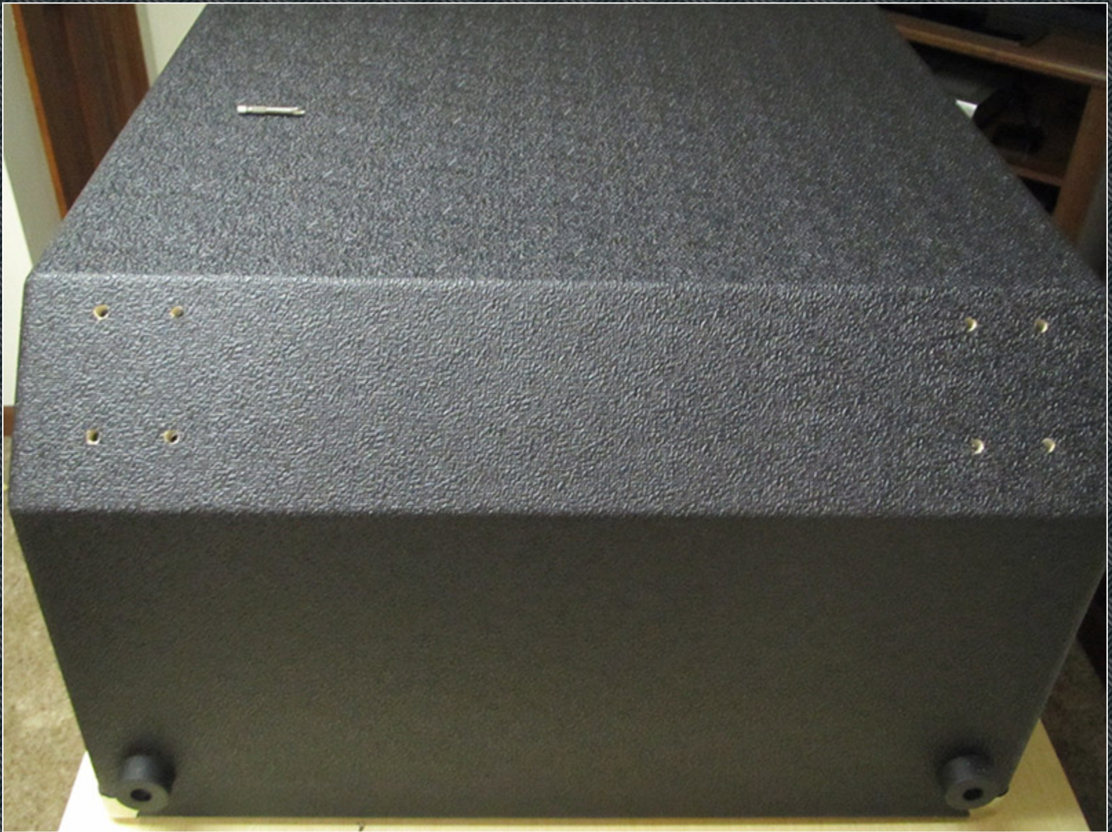
Drilling out the Tolex covering the caster mounting holes.
