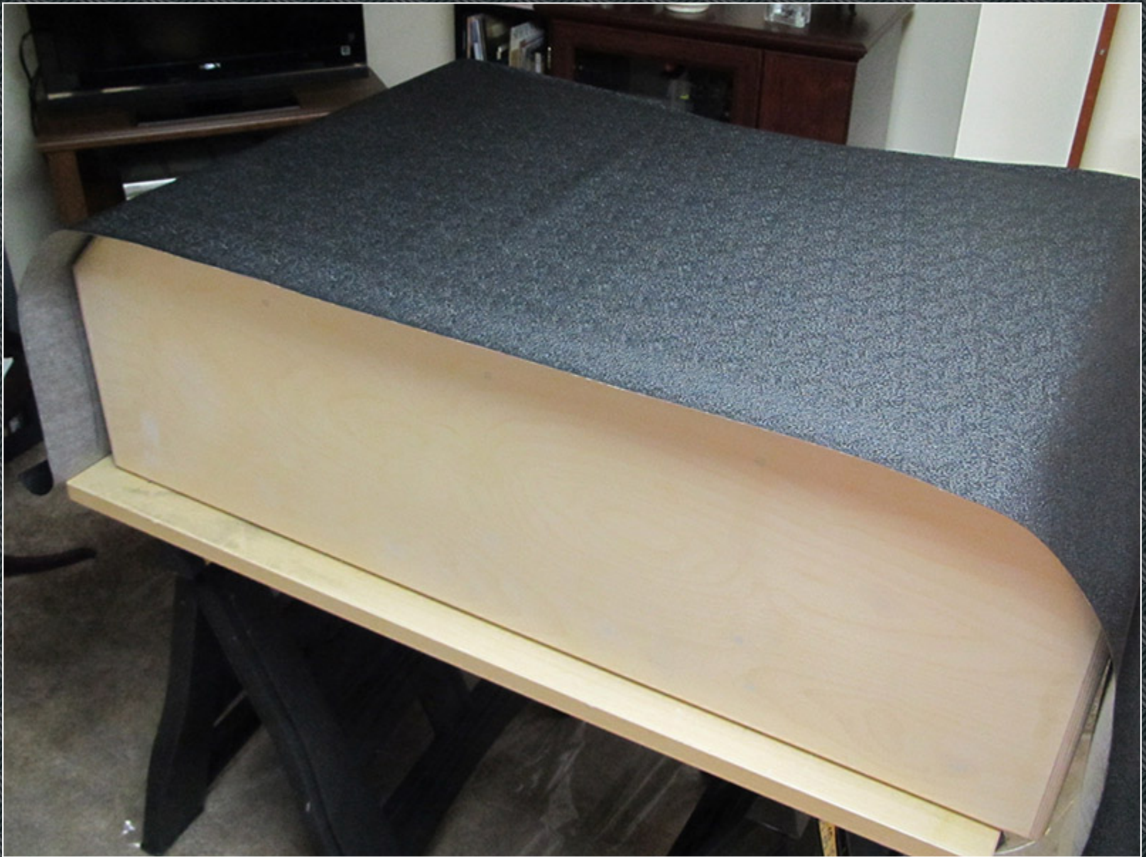
The back piece laying loosely on the cabinet so I can mark the edges on it.
