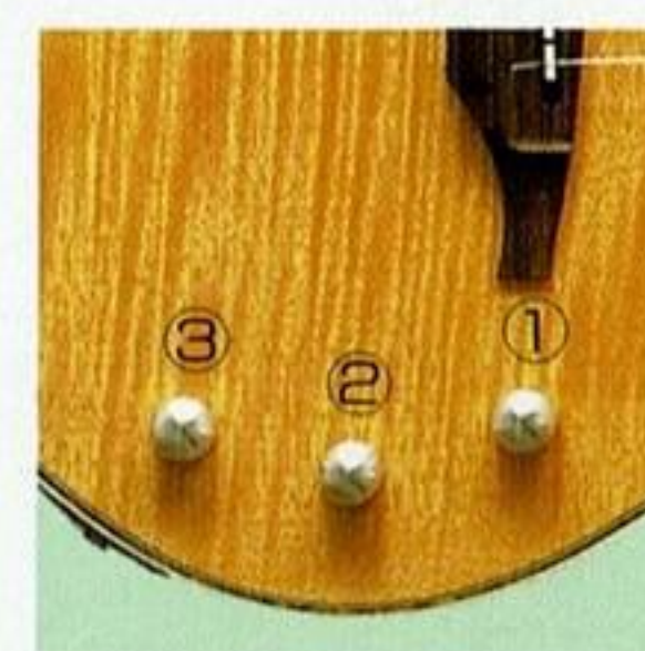
(TGX-823/812 Controls) 1. Pickup selector switch 2. Master volume 3. Master tone 4. 3way selector switch (Active 1, passive, Active 2)
